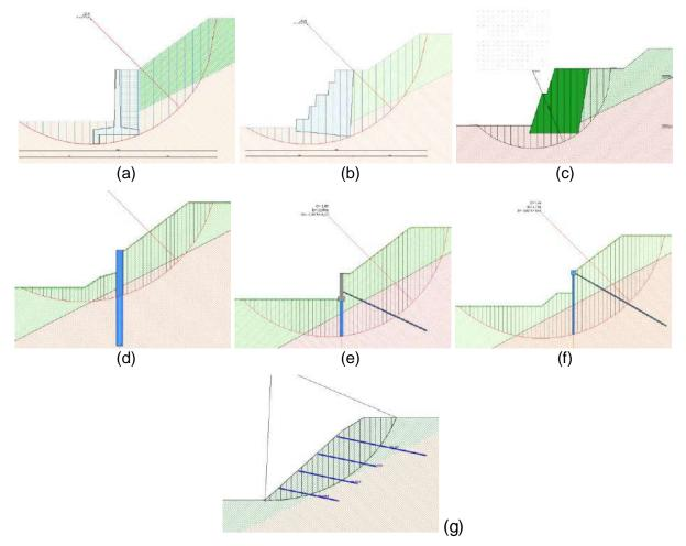
Figure 7. Interventions for the reference case: cantilever concrete retaining wall (a); gabion retaining wall (b); reinforced earth wall (c); line of drilled piles (d); tie-back micropile wall (e); tie-back wall with micropile (f); soil nailing (g).
